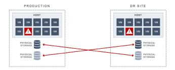
Figure 5. Mirroring systems over a fast network enables a very high availability, but corrupted software components are replicated as well.
