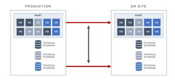
Figure 4. Array- and appliance-based replication methods require coordinating two replication products, one for the physical environment and another for the virtualized environment. This increases management complexity and undermines the investment made in virtualization.
